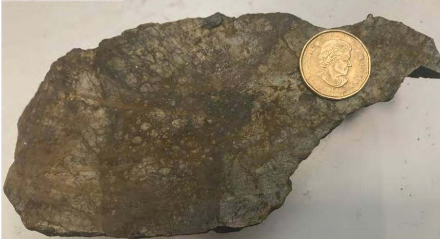
Channel sample A0600618 grading 19.24 g/t Au Eq including 4.75 Au Eq over 6.1m from the Lower Central Surebet Zone which remains open.
