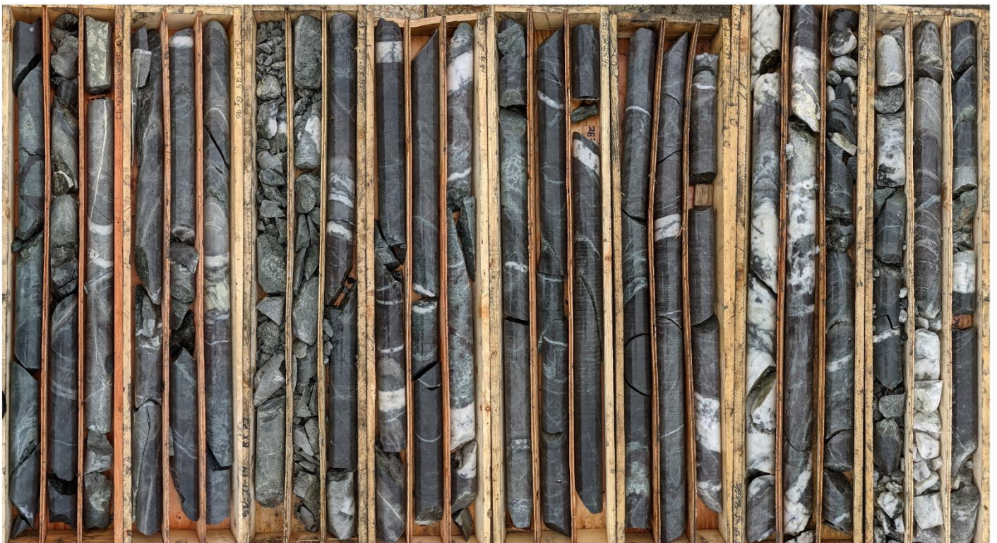
Real Deal GD-21-024, 273.72-295.44 meters (21.72 meter* intercept) of extensive veining and brecciation with sulphides of up to 10%. A 1,000 meter down dip extension of the Surebet Zone.
