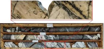
Pad A: Hole GD-22-39 from New Extension Target 81.89 – 87.01m: mineralization throughout unit consisting of trace disseminated galena, sphalerite and chalcopyrite, and interstitial to semi massive pyrrhotite, up to 10% locally
