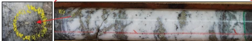
GD-23-183 - 472.75 - 477 m - Quartz vein with visible gold, galena, sphalerite, pyrite and pyrrhotite, hosted in Lower Hazelton Volcanics. Sample E080364 475 - 476 m
