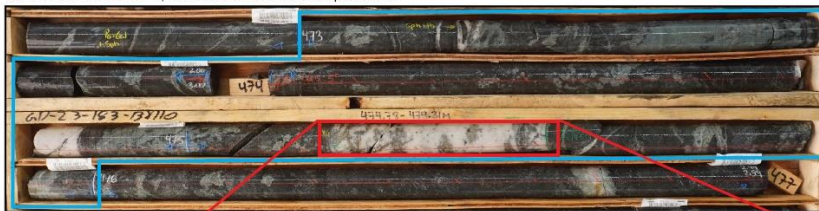
GD-23-183 - 472.7 - 477 m, Lower hazelton volcanics with quartz veins.
