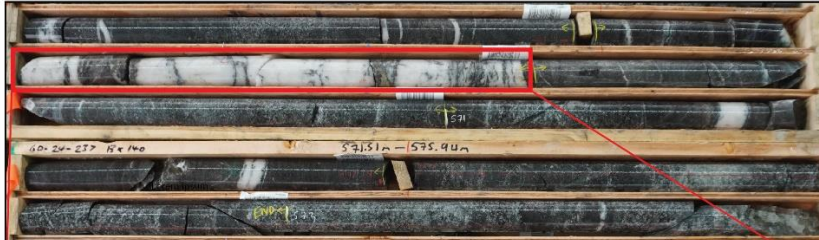
GD-24-237 - 568.90 - 573.85 m - Quartz vein with visible gold, galena, sphalerite, pyrite and pyrrhotite, hosted in Lower Hazelton Volcanics.
