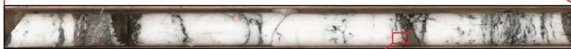
GD-24-237 - 569.29 - 570.04 m - Quartz vein with visible gold, galena, sphalerite, pyrite and pyrrhotite
