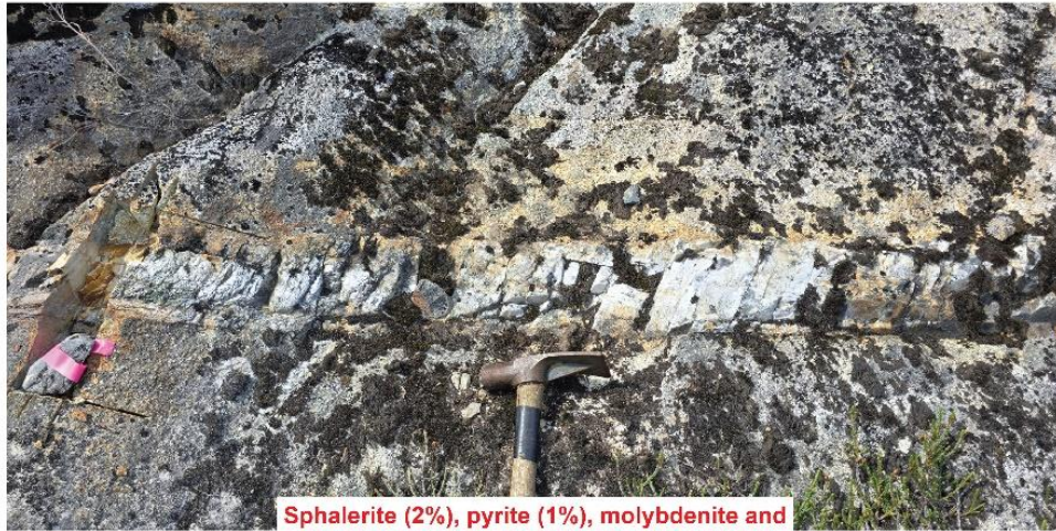
Sphalerite (2%), pyrite (1%), molybdenite and bismuth in 15 cm quartz vein crosscutting granodiorite pluton
