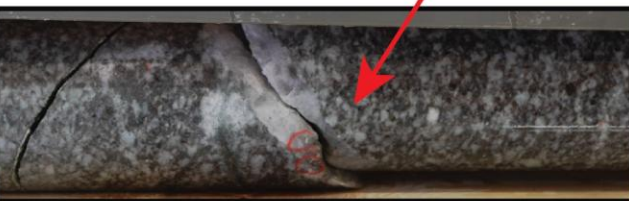
GD-24-237 - 316.28 m - Visible gold hosted within 12 mm quartz vein associated with native bismuth and molybdenite
