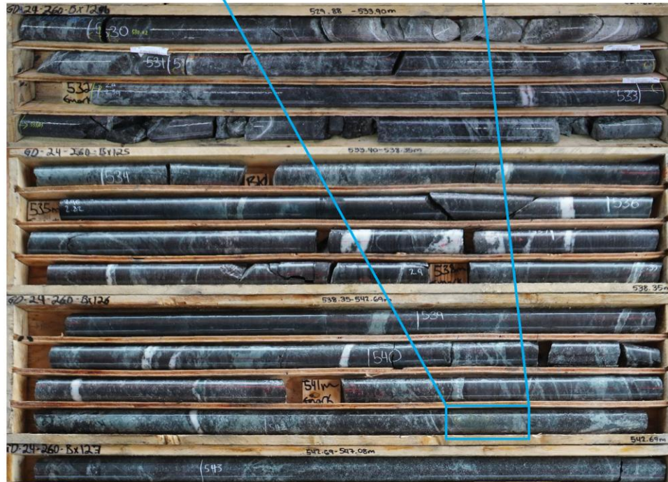
Bonanza quartz-sulphide veins in andesite hosting abundant visible gold, sphalerite, pyrrhotite and galena.
