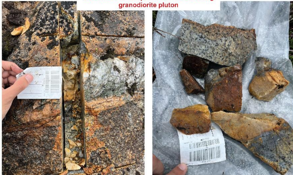
Sphalerite (2%), pyrite (1%), molybdenite and bismuth in 15 cm quartz vein crosscutting granodiorite pluton
