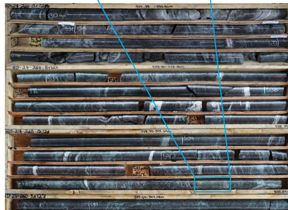
Bonanza quartz-sulphide veins in andesite hosting abundant visible gold, sphalerite, pyrrhotite and galena.
